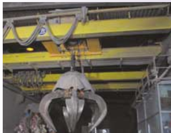
EOT double girder crane with one trolley application and hydraulic grab.
